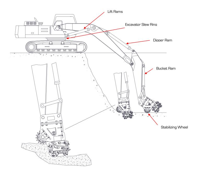
When the spoon cylinder is extended, the cutting unit is pressed into the ground, since the picks of the stabilizing wheel is supported in the ground.
